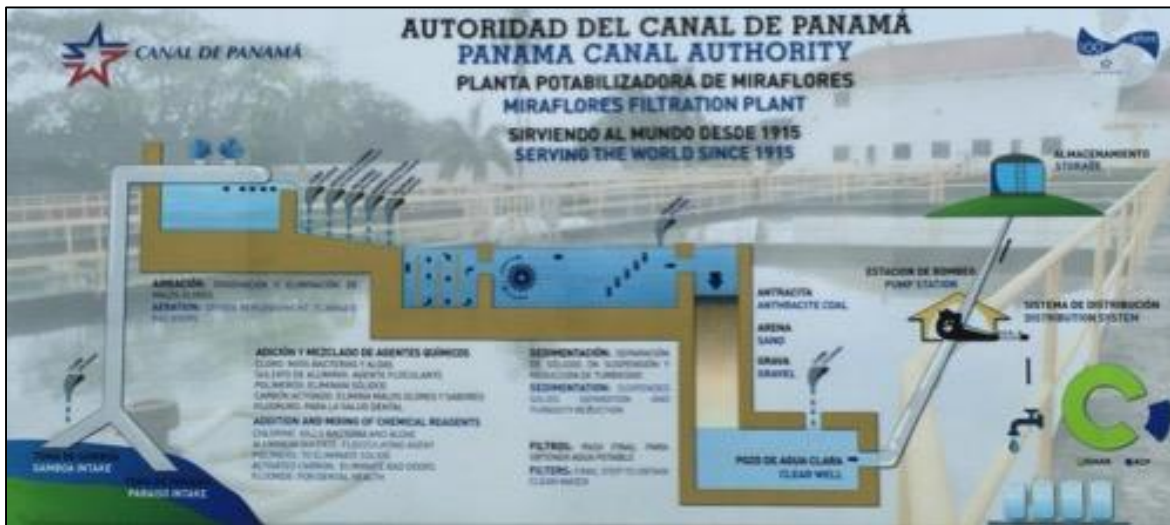
Figure 38: Water Treatment Process at the Miraflores Water Treatment Plant (Miraflores Water Treatment Plant, 2015)
