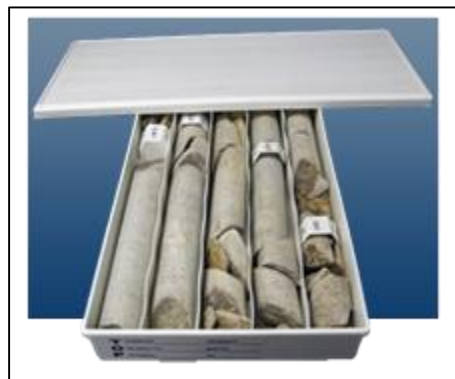
Figure 81: Example of core box (EVCO, 2015)
