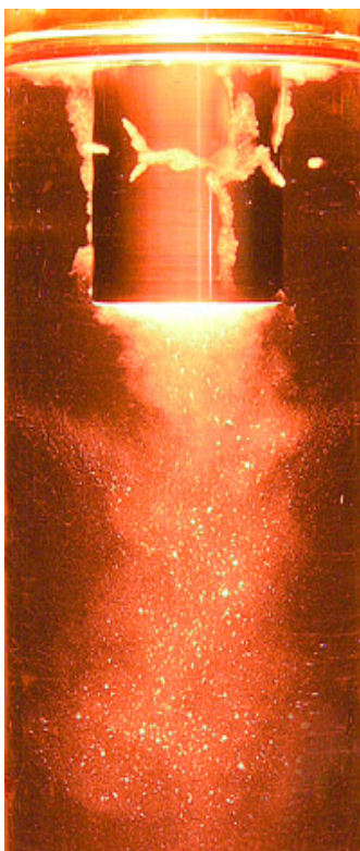
Figure 2.5.3: Ultrasonic cavitation for nanoparticle dispersion 36
