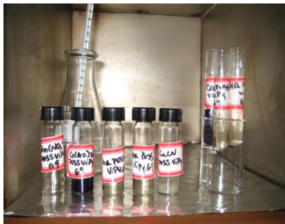
Figure 10. Experimental setup for the solvothermal synthesis of frameworks.
