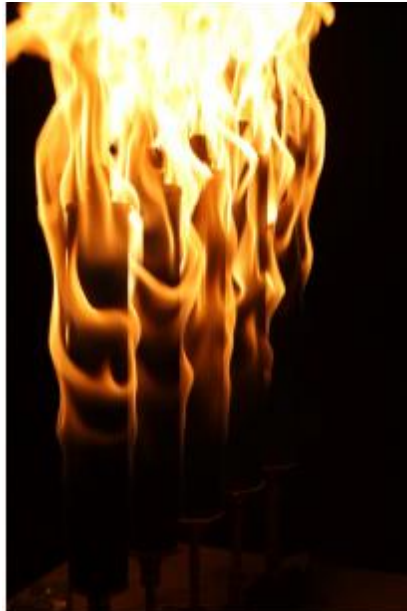
Figure 12 - Sample Flame of Cylindrical Port Burner
