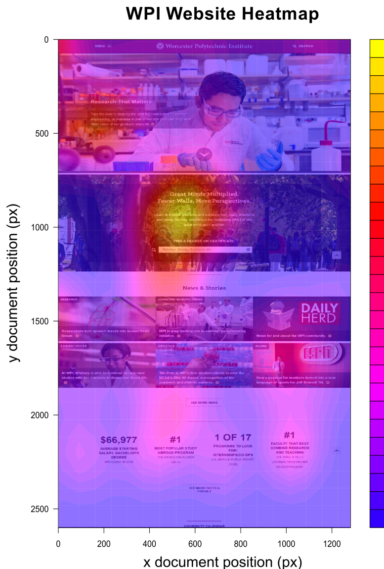
Figure 4.1: A heatmap of eye tracking data collected from EyeSite on a scrolling web page ( www.wpi.edu ). The only modification of the website's code was the inclusion of the EyeSite browser client script. Without taking special actions to avoid scrolling, this kind of visualization would be nearly impossible to make in other eye tracking frameworks.
