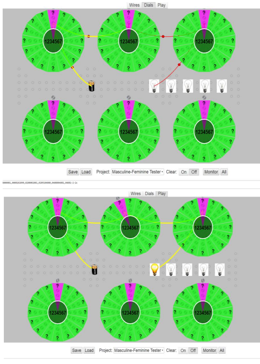
Figure 19. Example of “turning” a dial (middle top) to change the circuit state.
