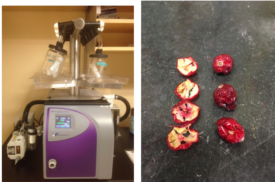
Figure 12: Bench-top Freeze Dryer and Photos of Lyophilized Cranberries
