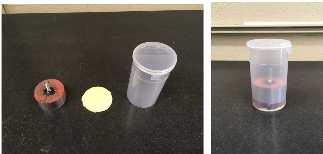
Figure 24: Components and Set-Up of the Syrup Expression Test
