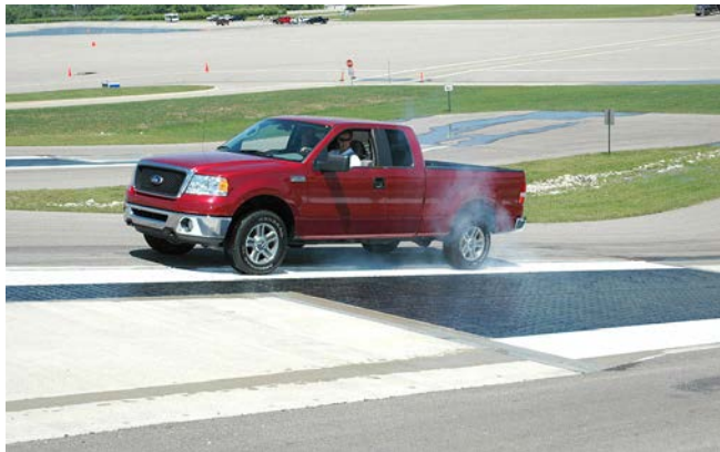
Figure 7 – Electronic Traction Control Testing
