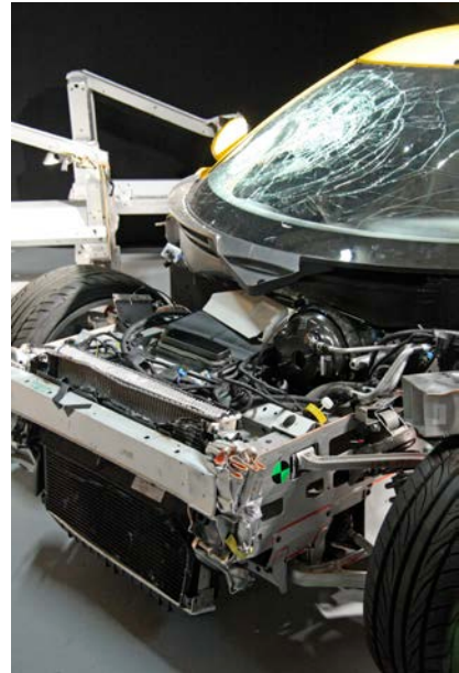
Figure 6 – Crumple Zone Testing
