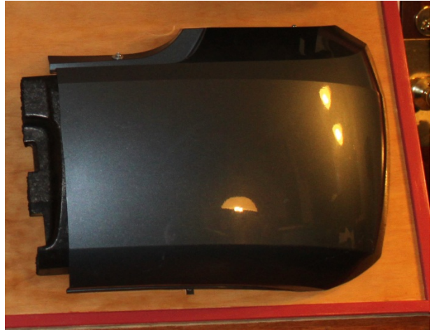
Figure 29 – Bumper Cut-Away (Crumple Zone)
