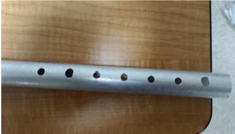
Figure 78: Main Shaft with Drilled Holes
