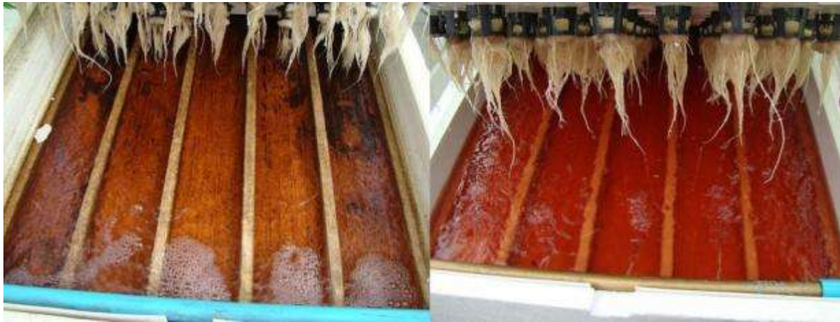
FIGURE 6: COMPARISON OF ALGAE GROWTH, VISIBLE AS BLACK RESIDUE, BETWEEN COMPARISON (LEFT) AND TRIAL (RIGHT) GROWING BEDS
