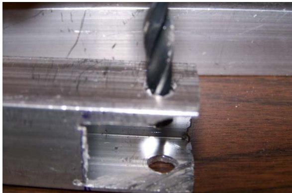
Figure 48 - Drilling joint holes
