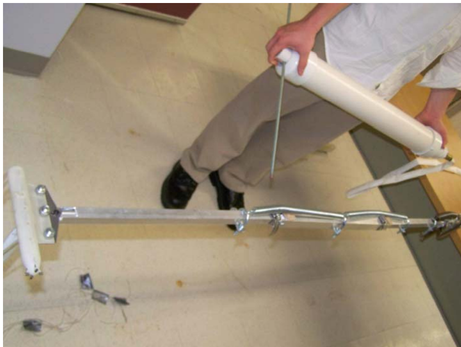
Figure 34 - Assembly extended: with the fire hose pressurized by the test pump, the arm is forced to extend, carrying the sensor package more than five feet away from its starting position.
