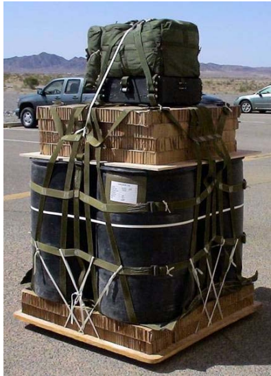
Figure 27 - A loaded Firefly 2k JPADS system, ready for drop 13
