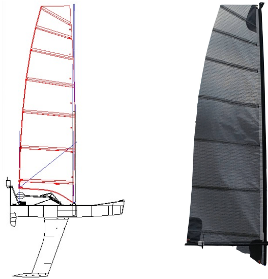
Figure 14: Design Drawing and Final Version of the Cloth Sail
