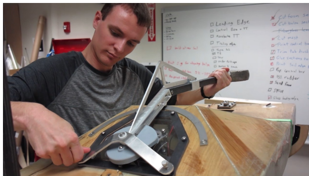
Figure 58: Hans Assembling the Movable Ballast for Testing
