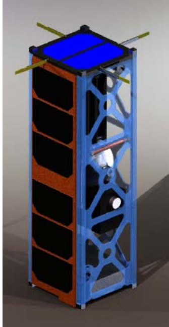
Figure 4 - Monoblock Design 2 (Assembly with Subsystem Components from 2010-2011 MQP) [2]
