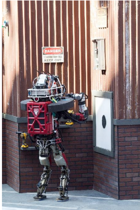
Figure 27: DRC Finals Drill task. Atlas preparing to pick up the drill. Note the sheetrock wall on the right.
