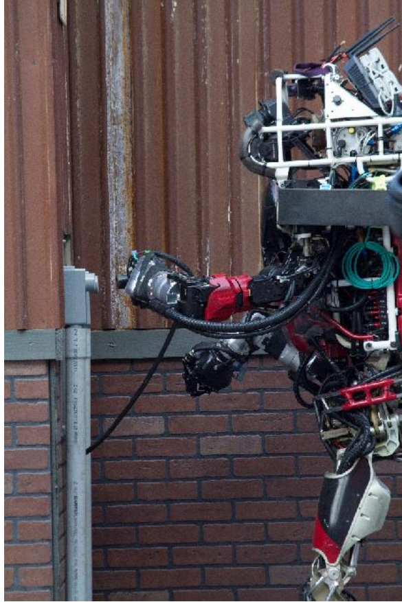
Figure 28: DRC Finals surprise task. Atlas is moving the plug from one socket to the other.
