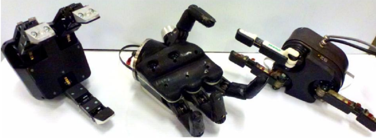
Figure 10: The three different hands the WPI-CMU DRC team tested. From left to right: Robotic 3 Finger Adaptive Gripper; Sandia hand; iRobot hand. The Robotiq hand was eventually selected for use.
