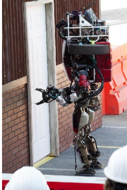
Figure 26: DRC Finals Door Task. Atlas reaching for the door.
