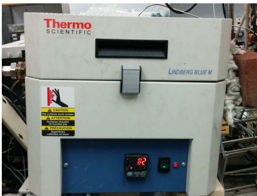
Figure 21: Lindburg/Blue tubular heater
