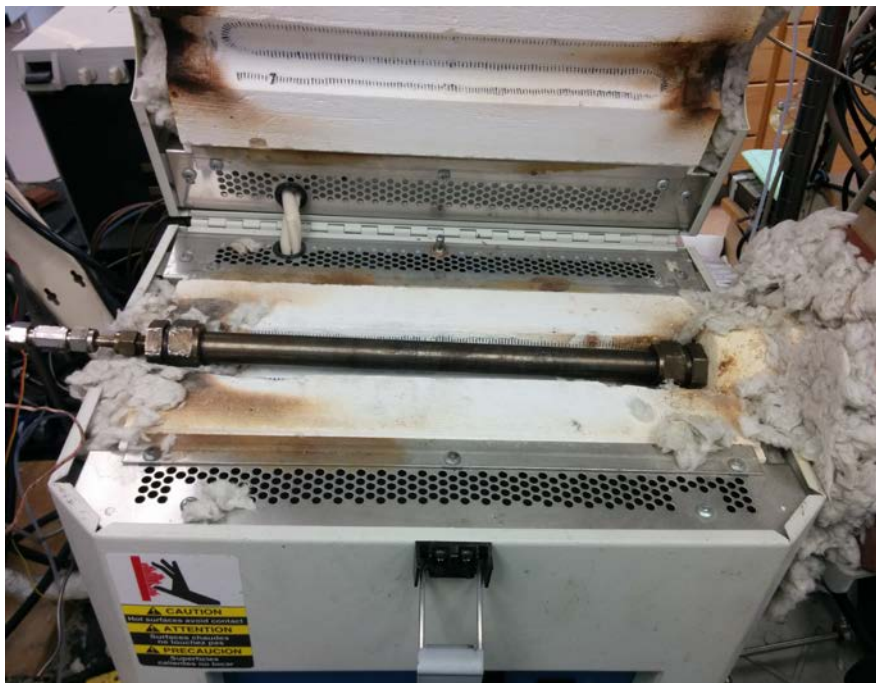
Figure 18: Reactor tube inside the furnace
