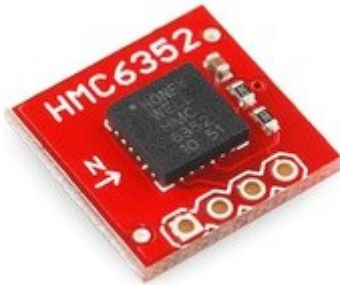
Figure 19 – Compass Module used as Navigation Aid (Sparkfun, 2013)
