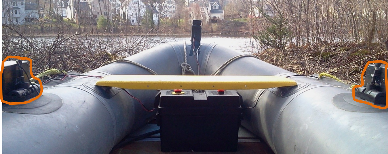
Figure 22 – TLD Mounting on the Rescue Craft – View from Stern
