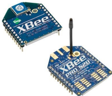
Figure 7 – XBee Ad-Hoc Network Device (Mouser, 2013)
