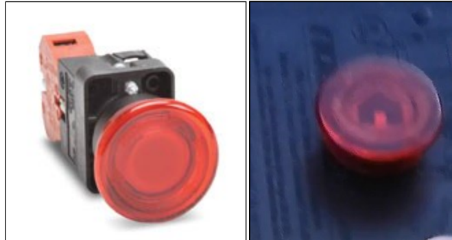
Figure 20 – Return Home Button on the Rescue Craft (automationdirect, 1999-2013)
