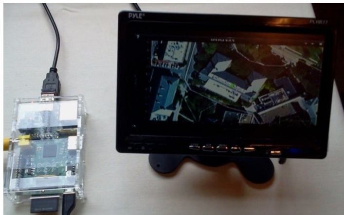
Figure 6 – Mothership Module Raspberry Pi and Pyle Monitor
