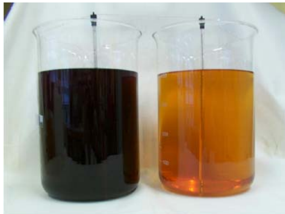
Figure 3: 70% color reduction of paper mill effluent achieved using the TAML ® activator and hydrogen peroxide.
