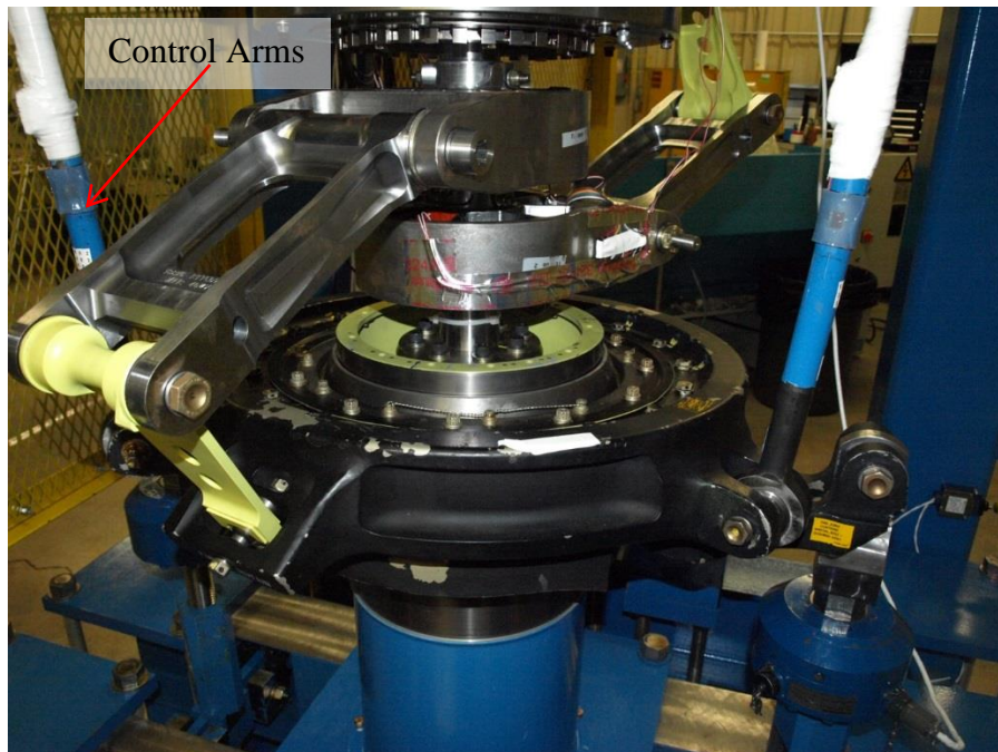
Figure 28: The scissor link from the University of Dayton Research Institute (University of Dayton Research Institute, 2014).
