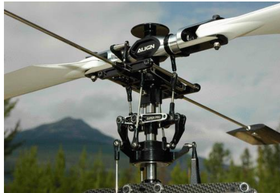
Figure 1: This figure depicts a Flybar Rotor Head (Salt, 2014)
