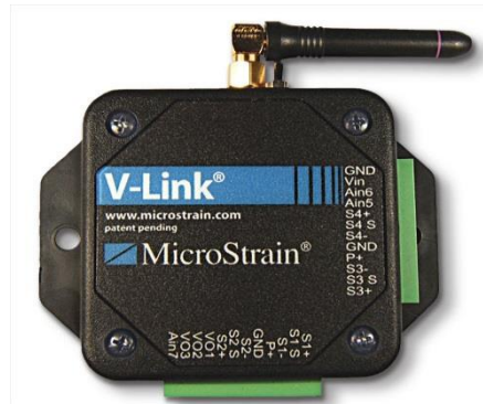
Figure 8: An example of a wireless strain gauge. (Lecklider, 2008)
