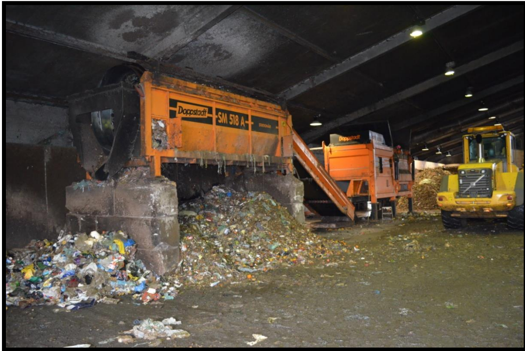
Figure 17: BioVækst's system for filtering plastic impurities
