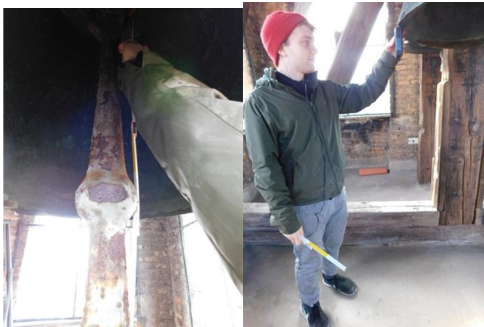
Figure 26 - Left: measuring the clapper length Right: measuring height from ground
