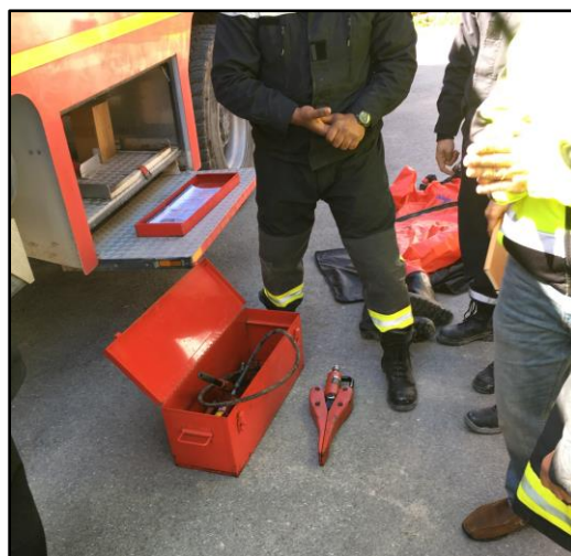
Figure 47: Hydraulics firefighters use if a person is stuck in or under a crashed vehicle
