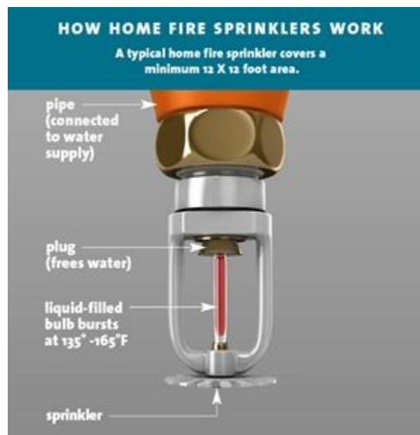
Figure 2: How Home Fire Sprinklers Work (NFPA, N.d.).
