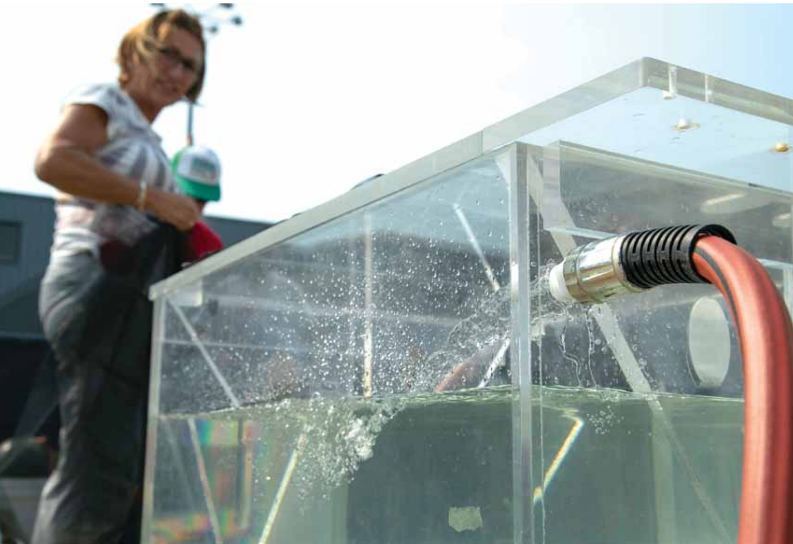
Plumbing the deck-board incubators to get them ready for measurements of phytoplankton growth and mortality.
