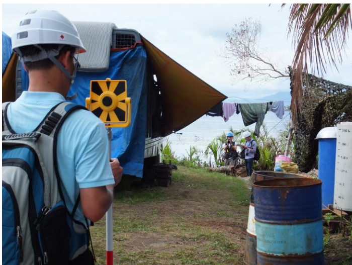
Figure 5 Use of a hand-held laser distance meter and target prism to conduct land surveys
