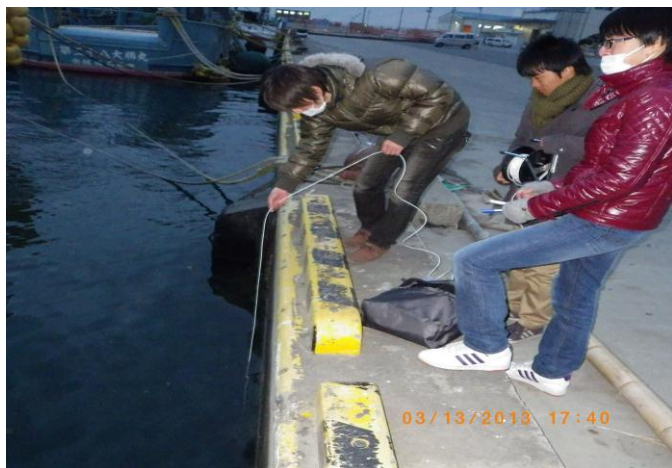
Figure 2 Rope with sensor attached to it to determine water depth
