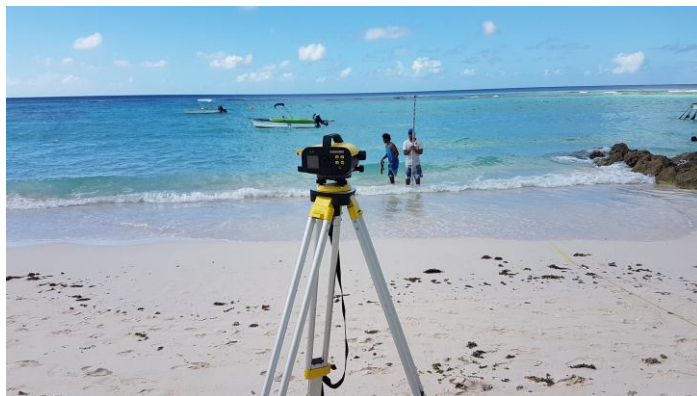
Figure 7 Measuring Procedure using a tripod and staff
