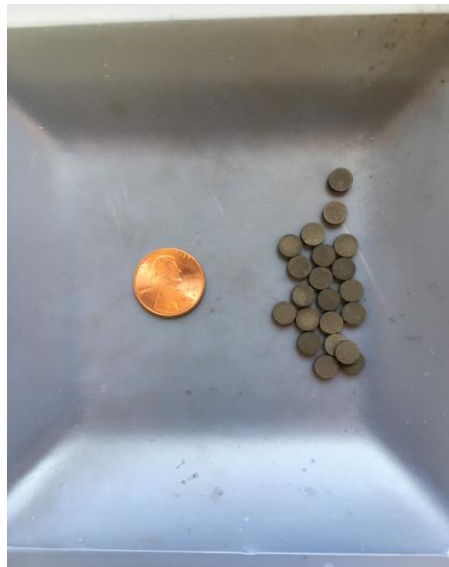
Figure 4: St171 sintered getter pellets by SAES Getters Group beside a US one-cent coin for scale.
