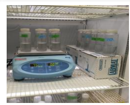
Experimental setup: incubation bottles on a shaker table (left) and on an elevated surface (right) to simulate turbulent and still condition, respectively.
