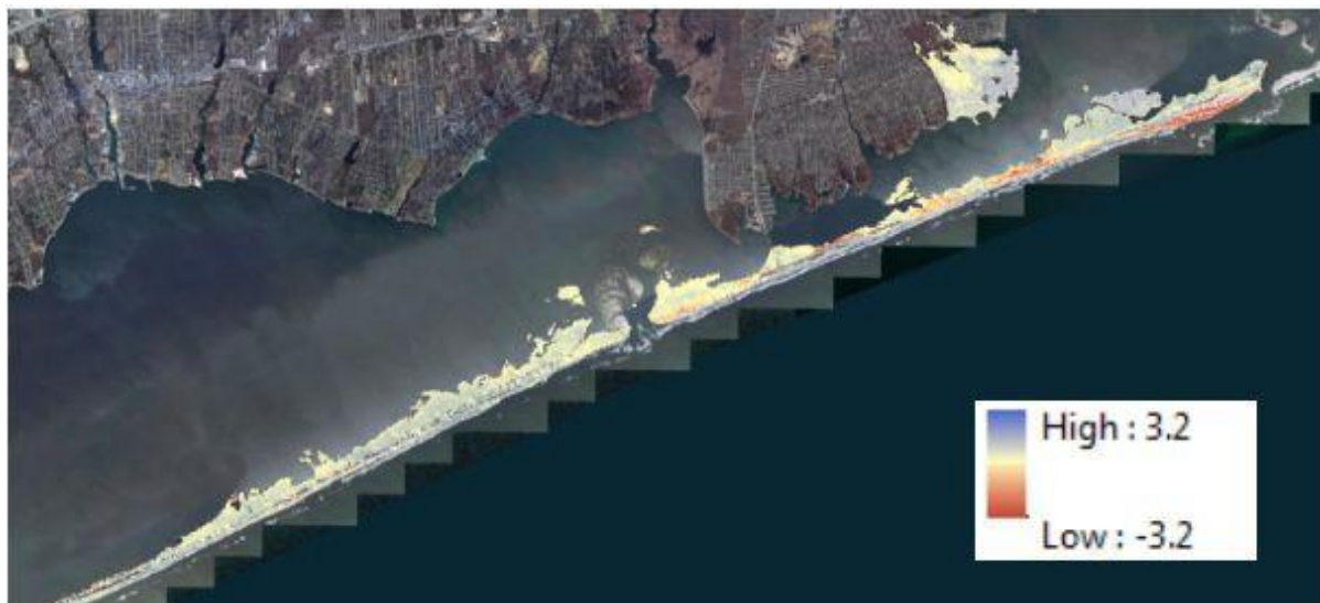
Fig. 9. Inundation depth differences for FIIS. Different gradients of blue represent areas where the Sandy Study projected deeper inundation, and the red areas represent where the Service Wide Study projected deeper inundation.
