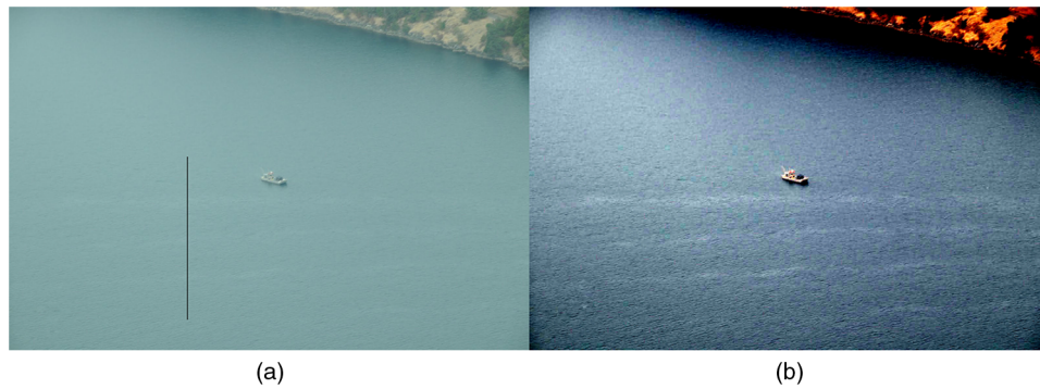
Fig. 10 Photo of the surface signature of one of the observed internal waves: (a) original with a black line marking the section plotted in Fig. 11; (b) same image after contrast enhancement.
