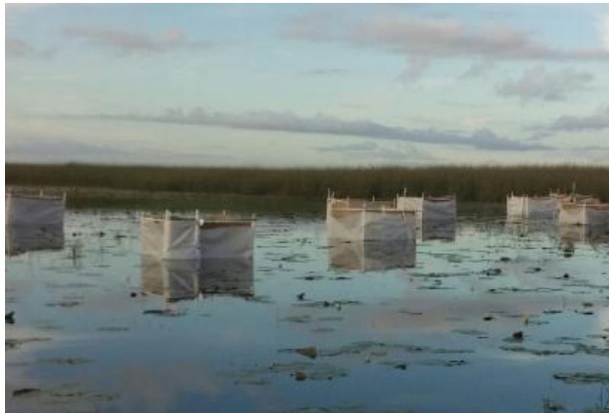
Figure S.4.2. (a) Photo showing mesh cages in the field. (b) Photo showing cages wrapped with 3mm clear plastic following nutrient dosing. Phosphorus ( \text{Na}_2\text{HPO}_4 ) was added once per week and the cages remained wrapped for 24 hours to avoid seepage to cages without nutrient addition.
