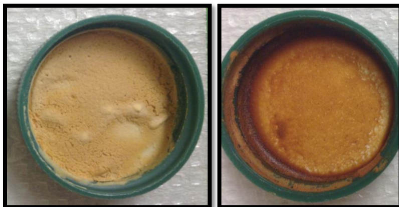
Figure 14 - Dried discs samples for IAEA-153 and IAEA-155 after addition of internal standard and 0.5mL of water and drying overnight
