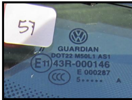
Figure 31 - An example of a window marking found on the windshield of a vehicle
