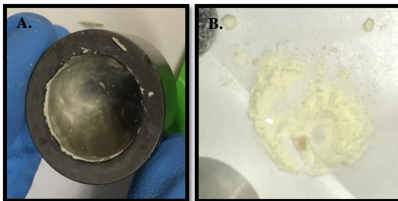
Figure 22 – A. Sample adhering to mill jar because the frequency was too high and/or the length of milling was too long B. Clumps of milk powder that were not milled long enough at a high enough frequency
