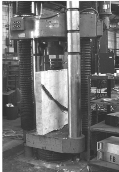
Figure 2-11: Testing of isolated strut specimen and the variables [5]
