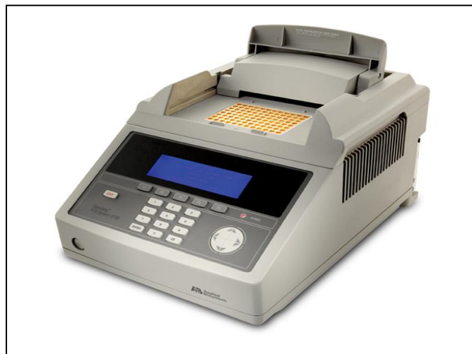
Fig.3.3 GeneAmp® PCR system 9700 thermal cycler from Life Technologies. Temperature ramp rate 4°C/s, fits 96 samples at once and has heated lid to prevent condensation. From Thermo Fisher Scientific website.
