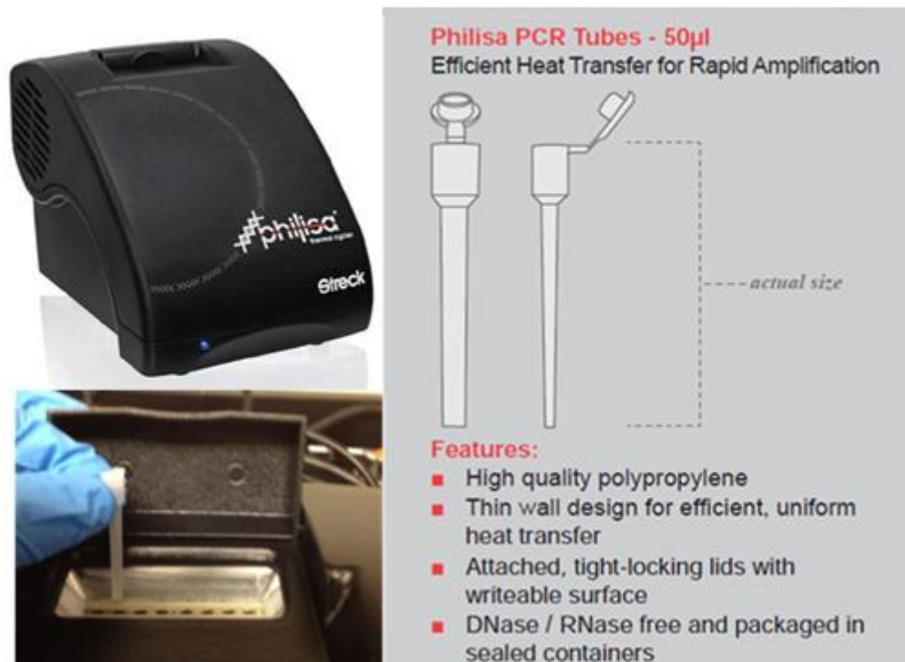
Fig.5.1 Philisa ultra-fast thermal cycler. Instrument shown top left. The silver heat block with PCR tube shown bottom left. Specially designed thin, flat PCR tube shown on right. The Philisa cycler is has heating rates of 15°C/s and 12°C/s cooling.
