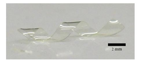
Figure 2.3. Example of a twisted nematic LCE actuating in response to heat.
