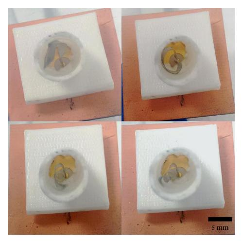
Figure 4.18. Dynamic prototype LCE Antenna inside the cylinder brace at different states: no turns at 25°C, 1-turn at 40°C, 2-turn helix at 63°C, and 3-turn helix at 80°C.
