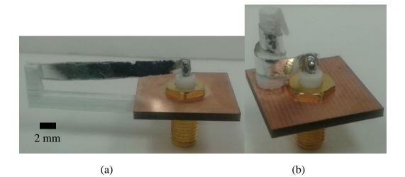
Figure 3.11. Static prototype of pattern-reconfigurable LCE antenna #1 at different states: (a) straight and (b) 1.1-turn spiral.
