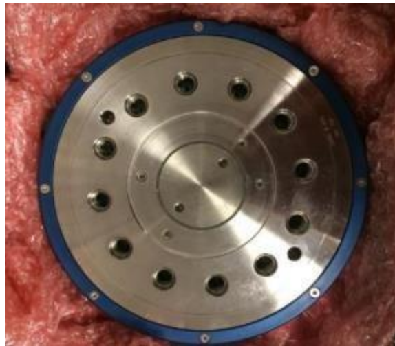
Figure 2-17 - 6 degree of freedom load cell
