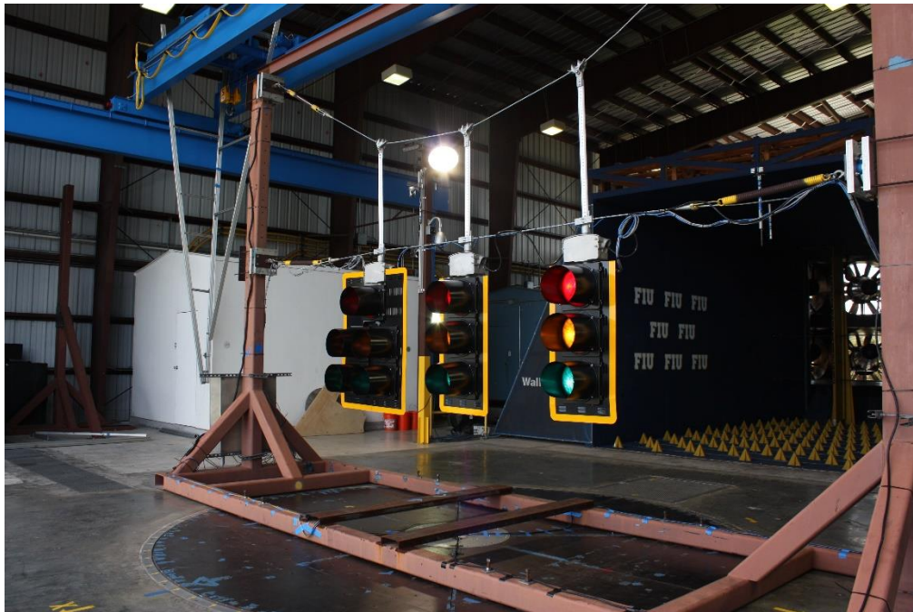
Figure 2-7 - Test rig with traffic lights assembly
