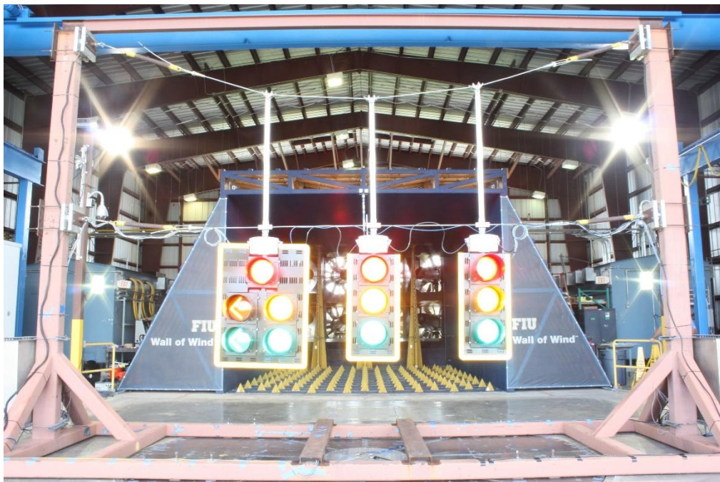
Figure 2-11 - Modified traffic light assembly (3% sag, 7 feet distance between catenary and messenger load cell, standard messenger wire pre-tension)
