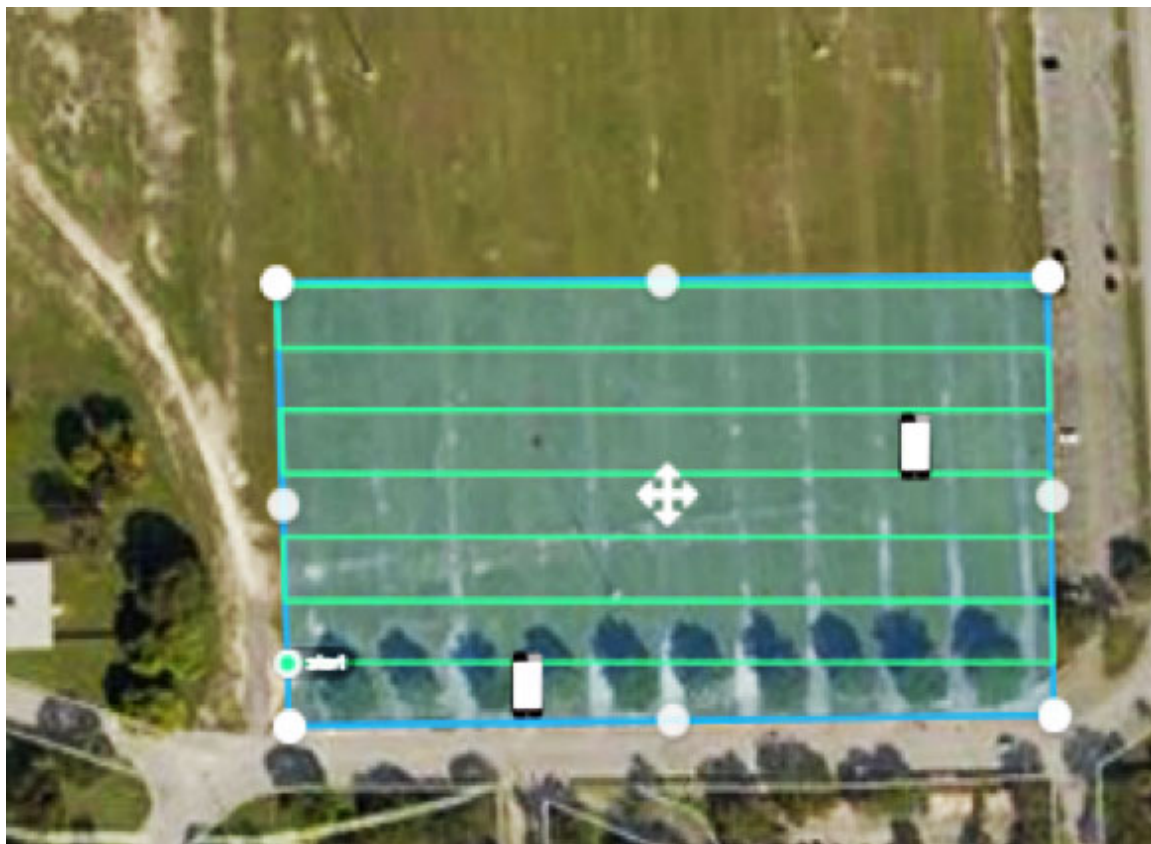
Fig. 10. Parallel Track Search Pattern traveled by the UAV.
