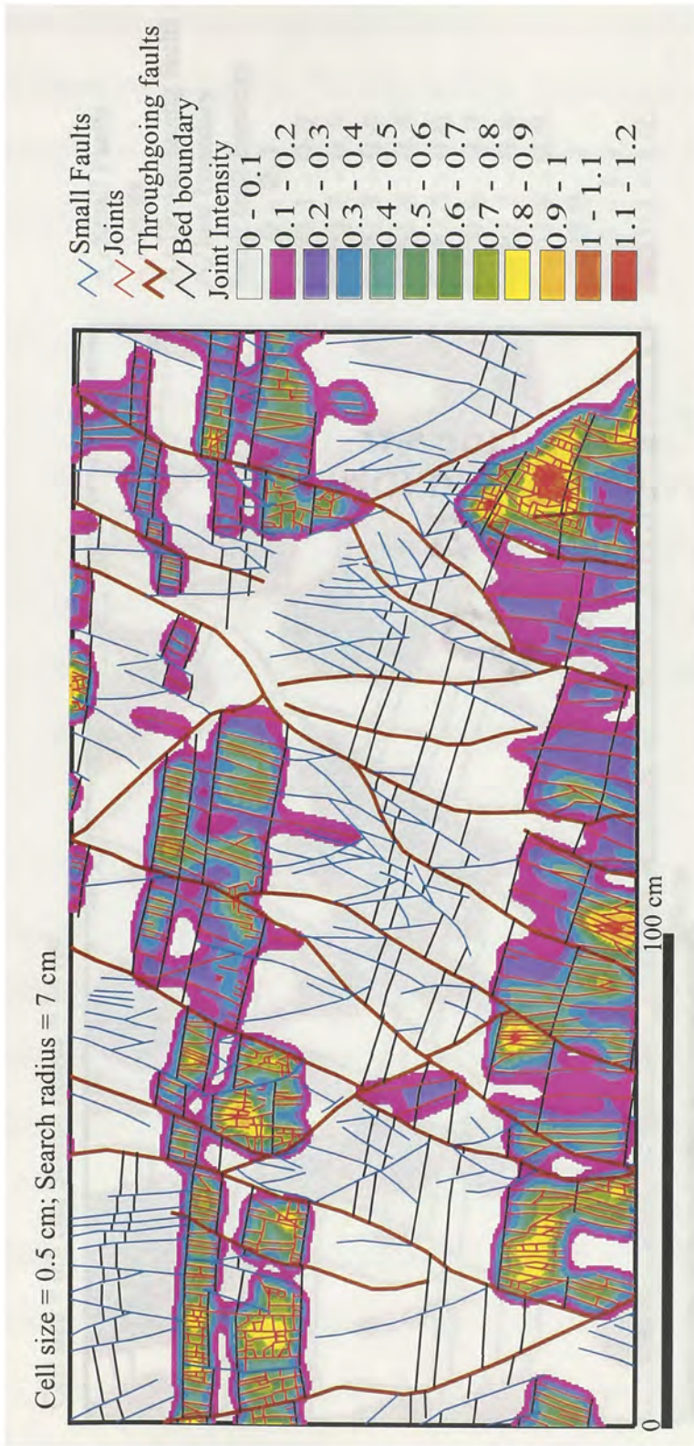
Fig. 4.5 Joint intensity map of Section 1. The mean joint intensity for the whole area is 0.14/cm and the average intensity in the porcellanite units is 0.35/cm.
