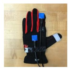
Figure 6.9: The glove with IMUs attached on the back of the hand and on the tip of index finger
