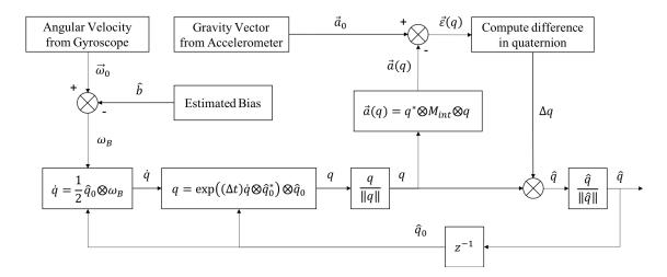
Figure 6.1: Block diagram of the orientation correction algorithm using only gravity vector correction
