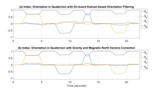
Figure 6.12: The plots of estimated quaternion results (a) with On-board Kalmanbased Orientation Filtering and (b) with gravity and magnetic North vectors correction for IMU attached on the index finger
