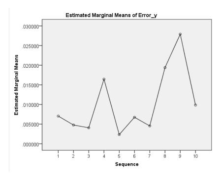
Figure 8.5: Estimated marginal means of the position errors in y
