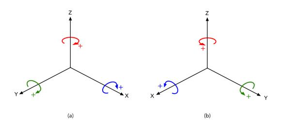
Figure 2.1: (a) Left-hand coordinate system and (b) right-hand coordinate system
