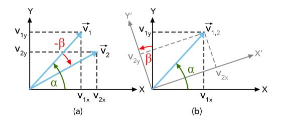
Figure 2.4: Difference perspective of rotation on XY-plane (frame rotation)
