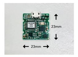
Figure 5.8: Yost Labs 3-Space<sup>TM</sup> micro USB
