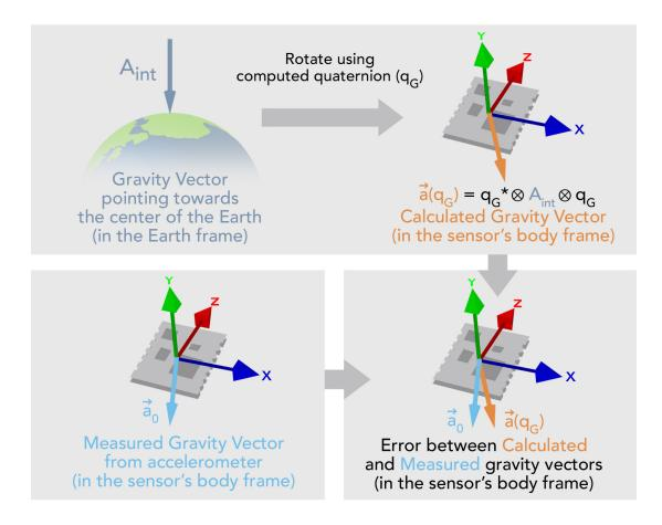
Figure 4.2: Quaternion correction using the gravity vector
