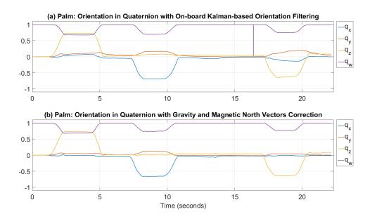
Figure 6.11: The plots of estimated quaternion results (a) with On-board Kalmanbased Orientation Filtering and (b) with gravity and magnetic North vectors correction for IMU attached on the back of the hand
