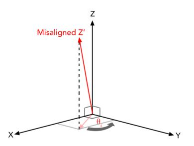
Figure 3.5: Misalignment or axes non-orthogonality errors
