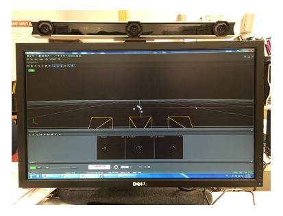
Figure 5.2: The setup of OptiTrack V120: Trio with Motive:Tracker software running on the host PC
