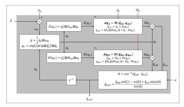
Figure 4.1: Block diagram of the proposed drift correction algorithm using both gravity vector and magnetic North vector correction
