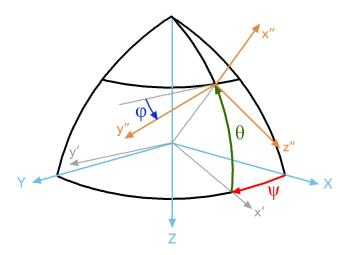
Figure 2.5: The aerospace Euler angle-axis sequence
