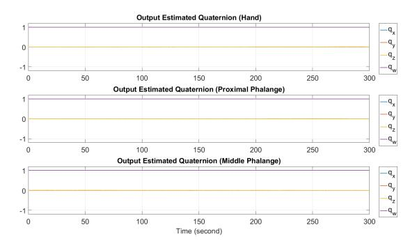
Figure 7.6: Output estimated quaternions with orientation correction algorithm
