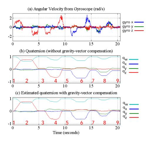
Figure 6.6: (a) Angular Velocity, (b) Quaternion without gravity vector compensation, (c) Estimated quaternion with gravity vector compensation
