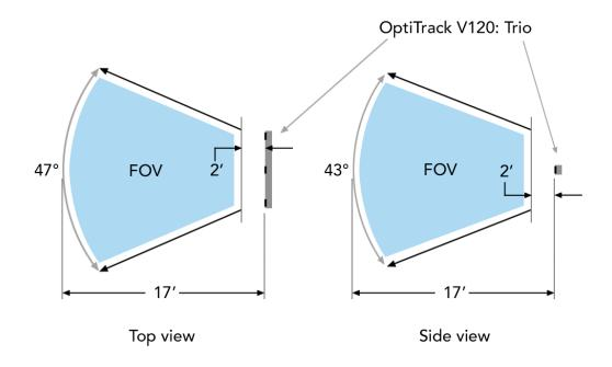
Figure 5.3: The field of view (FOV) of OptiTrack V120: Trio
