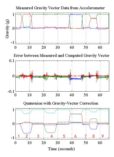
Figure 6.4: The plots of measured gravity vector from accelerometer, error between measured and computed gravity vector, estimated quaternion result (with gravity-vector correction). The numbers written at the bottom of the lower plot identify 9 "poses" or "stages" in which the module was held temporarily static.
