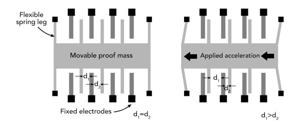
Figure 3.1: Mechanical structure of MEMS accelerometer
