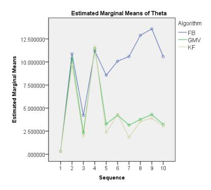
Figure 8.8: Estimated marginal means of the orientation errors for Theta
