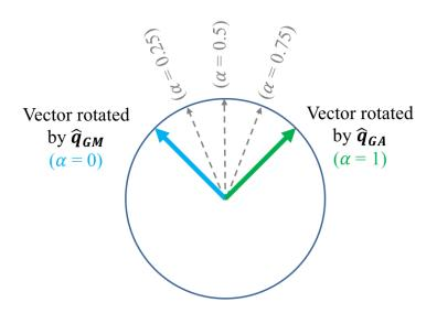
Figure 4.4: Spherical linear interpolation between  $\hat{q}_{GM}$  and  $\hat{q}_{GA}$
