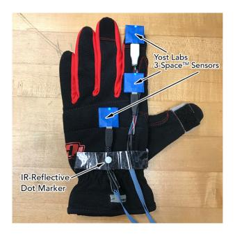
Figure 5.4: The glove with IR-reflective dot markers attached on the wrist, one Yost Labs 3-space sensor attached on the back of the hand, and two Yost Labs 3-space sensors attached on the index finger
