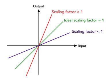
Figure 3.4: Scaling factor errors
