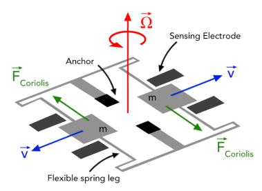
Figure 3.3: Coriolis effect in vibratory MEMS gyroscope
