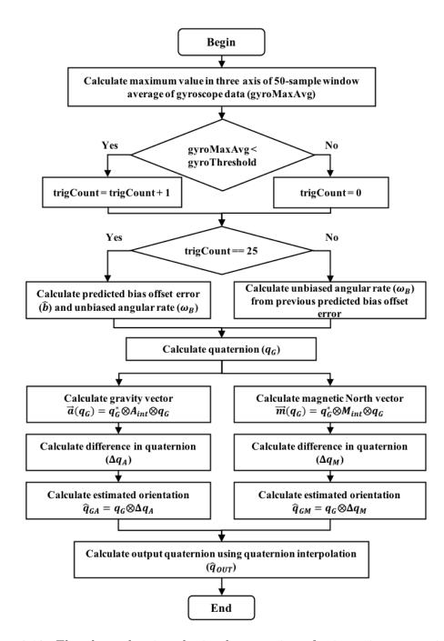
Figure 6.10: Flowchart showing the implementation of orientation correction algorithm for one iteration using both gravity and magnetic North vector corrections
