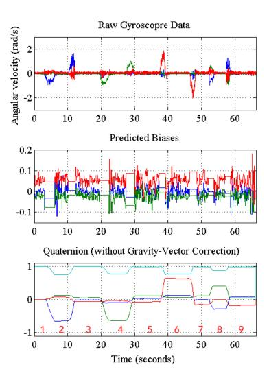
Figure 6.3: The plots of raw gyroscope data including bias offset error, predicted bias error, quaternion result (without gravity-vector correction). The numbers written at the bottom of the lower plot identify 9 "poses" or "stages" in which the module was held temporarily static.
