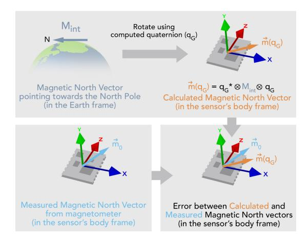
Figure 4.3: Quaternion correction using the magnetic North vector
