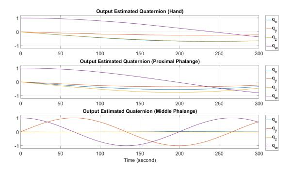
Figure 7.5: Output estimated quaternions without orientation correction algorithm
