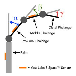
Figure 5.9: Finger joint angles and position of Yost Labs 3-Space<sup>TM</sup> sensors
