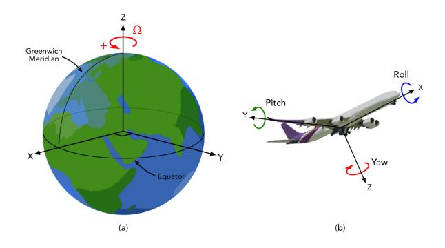
Figure 2.2: (a) Earth frame and (b) body frame
