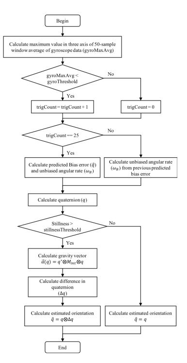
Figure 6.2: Flowchart showing the implementation of drift correction algorithm using only gravity vector compensation for one iteration with the condition that the module should be in a static period (Stillness)
