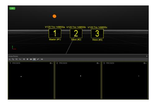
Figure 5.5: Visible dot marker on three infrared cameras (white dots) and position of the marker in 3D space shown as an orange dot
