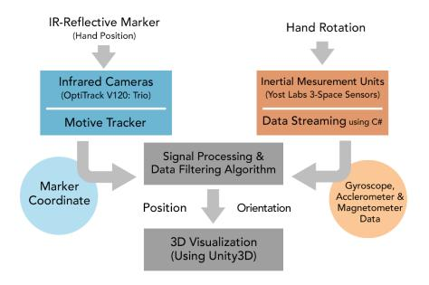
Figure 5.1: Overview of hand motion tracking system using inertial measurement units and infrared cameras
