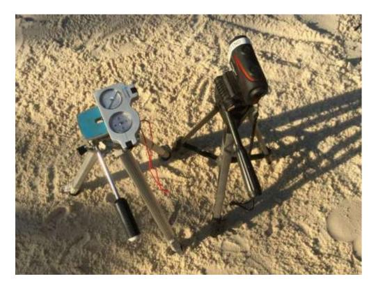
4-1. The Nikon Prostaff 7 Laser Rangefinder and Steren Electronics compass are mounted on a photographic tripod to measure the speed and path of a rip current. The speed is measured by calculating the distance with the laser rangefinder of a floating object moving inside the rip current over time. The compass is used to determine the angle of the rip path in order to correct the distance measurements for a non-linear rip current path.
