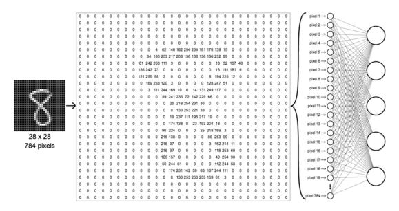
Figure 2.7: Encoding Image into Neural Network
