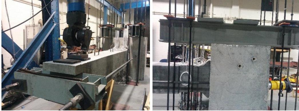
Figure 4-5 Loading setup and support conditions.
