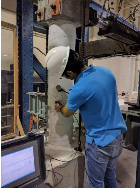
Figure 6-38 Measuring the mobility of the column.
