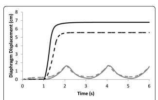
Figure 1 Diaphragm displacement during tidal breathing (grey lines) and maximal inspiration (black lines). Uninjured curves (solid lines) reproduce published experimental data. When simulating electrical stimulation (reverse recruitment) and fatigue (a 50% reduction in maximal muscle force), tidal breathing results are similar to uninjured simulations due to increased force generated by the larger motor units being recruited first (dashed lines).
