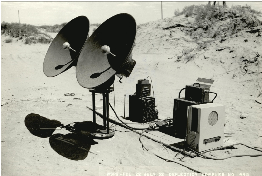
Figure 9. Doppler radar dishes with remote electronics at WSPG, 1952 (WSMR Museum Archives)
