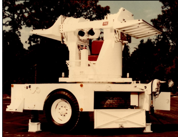
Figure 89. WSMR Lightweight Optical Tracking System (LOTS) (Bellinger Collection, WSMR Museum Archives)
