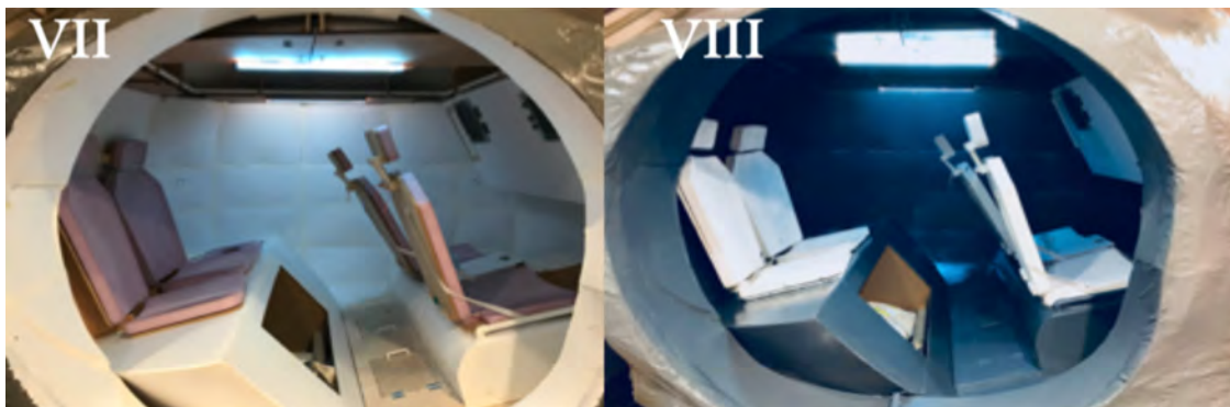
Figure 19: Interior of MAV simulates design for numerical results of Case 2 Brightness from an internal artificial light source.
