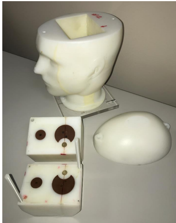
Figure 10: IROC-Houston's conventional H&N phantom is constructed using solid HIPS and is equipped with a centrally located single insert. The insert has two parts that combine to create an acrylic spinal cord, a semi-circle primary PTV and a circular secondary PTV constructed of solid water.
