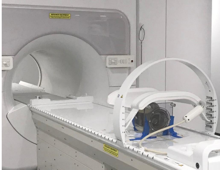
Figure 25: The MRgRT H&N setup at MD Anderson's Unity System. The MRgRT H&N phantom was secured in place with blue tape and a white foam coil was fastened above the phantom. The coil was used to capture an MR image and remained on during the irradiation. It should be noted that the coil was lowered close to the phantom's surface but did not directly contact the phantom.
