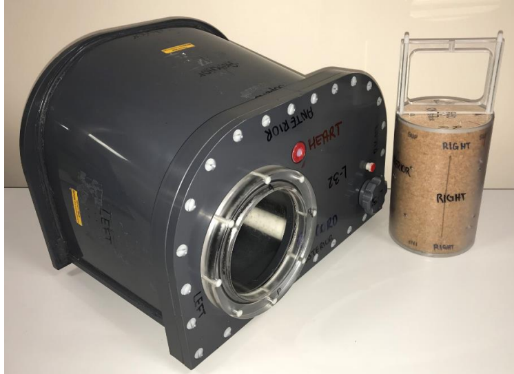
Figure 9: IROC-Houston's water-fillable anthropomorphic lung phantom contains a nylon heart, an acrylic spinal cord, two compressed cork lungs and a centrally located HIPS tumor inside the left-side lung. The left-sided lung is created from an external insert that is mounted to a motion table to simulate breathing.
