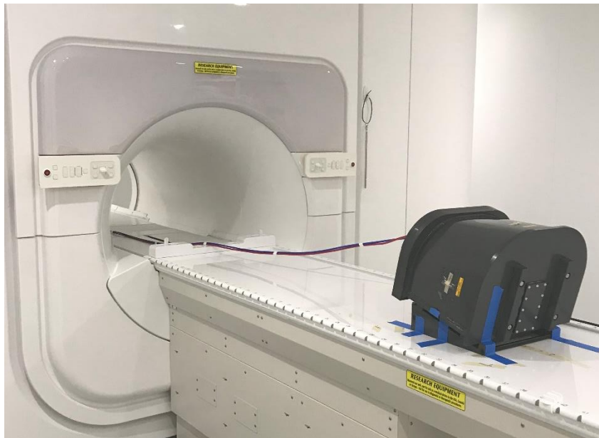
Figure 31: The MRgRT Thorax Phantom setup up for the reproducibility study. The MRgRT body coil was used to capture an MR image.
