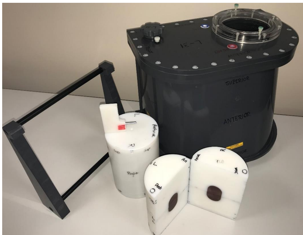
Figure 28: The MRgRT Thorax Phantom. The phantom consists of a water-fillable anthropomorphic thoracic shell, an inclining 15-degree platform and an external insert shell that holds four individual MR/CT compatible insert pieces.
