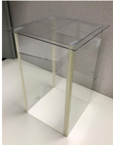
Figure 1- Assembled irradiation stand and platform for mouse phantom
