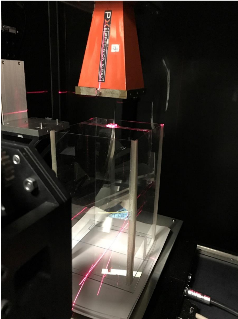
Figure B-3. Experimental setup for irradiating thermoluminescent dosimeters in-air
