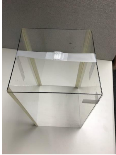
Figure 2- TLD capsules secured to irradiation stand.
