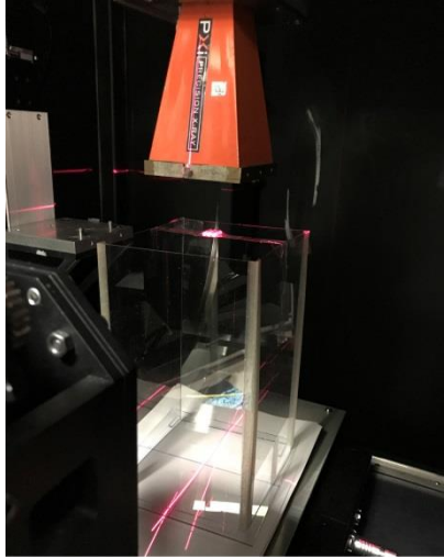
Figure 4- Setup for in-air TLD irradiation
