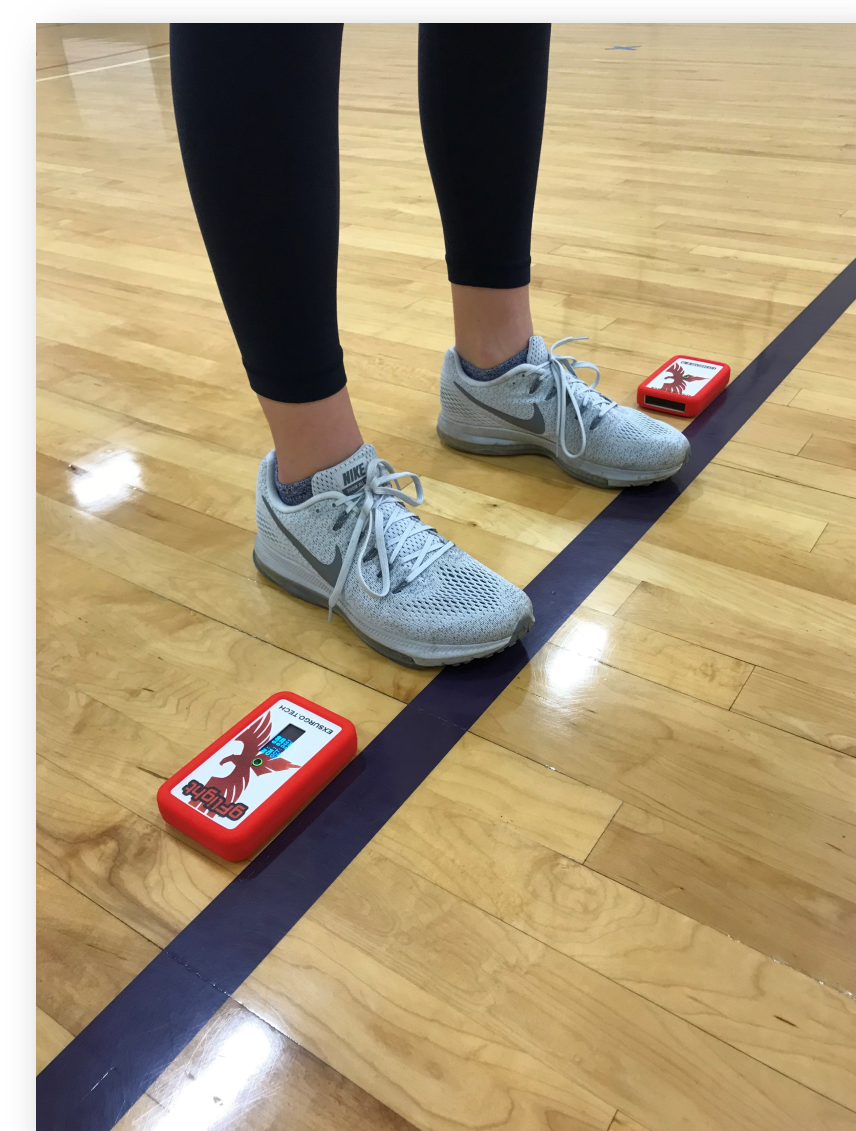
Figure 3: Proper set-up for using the gFlight for jump testing. Connected via Bluetooth to an iPad.
