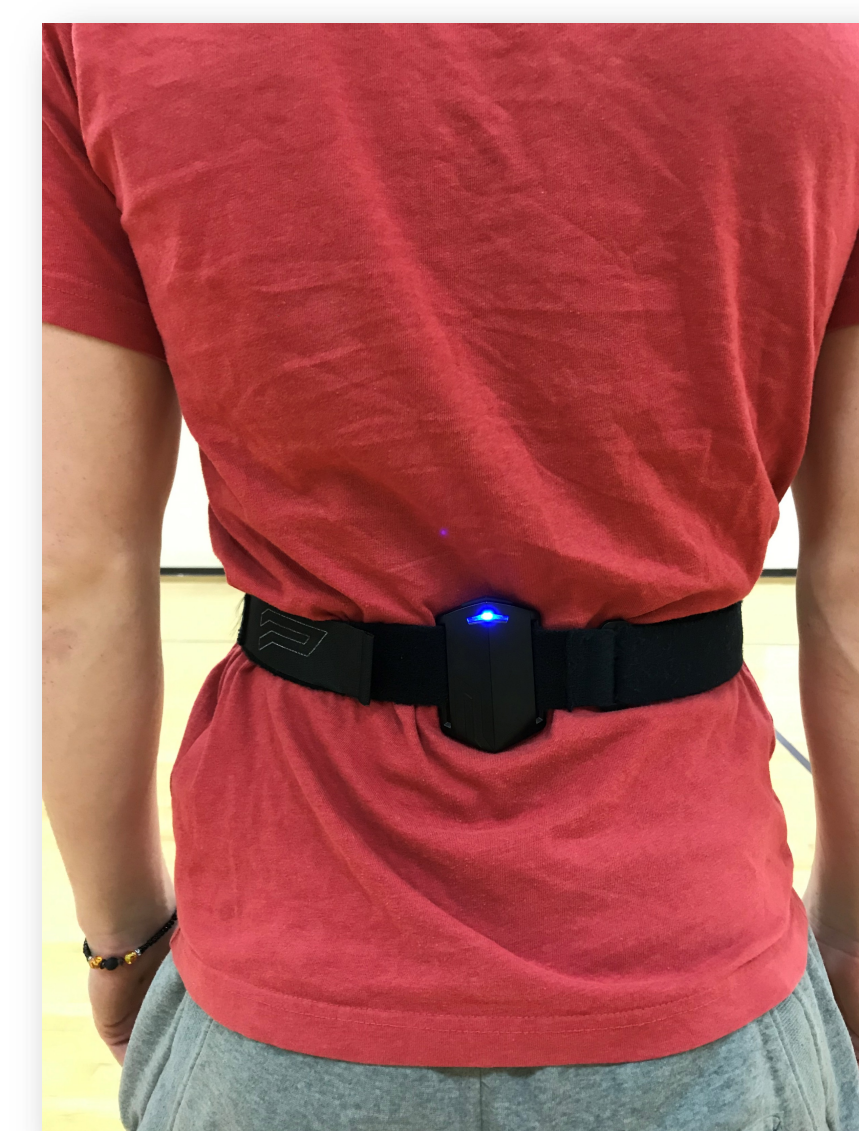
Figure 2: The correct placement of the PUSH Band sensor for jump testing. Connected via Bluetooth to an iPad.
