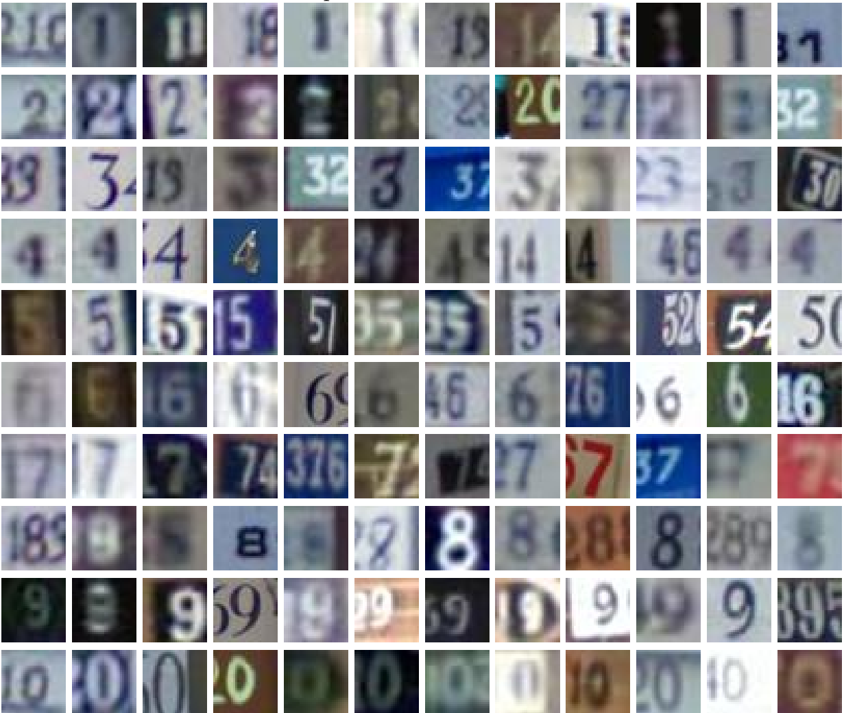
Figure 4.7: Sample from SVHN dataset. SVHN dataset compiles images from 10 different classes. All images are colorful and of the size 32 \times 32 .
