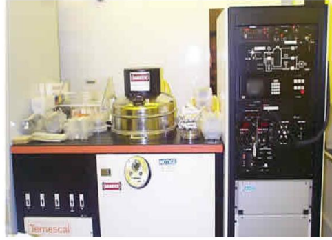
Figure 2. 8. BJD 1800 e-beam metal evaporator.
