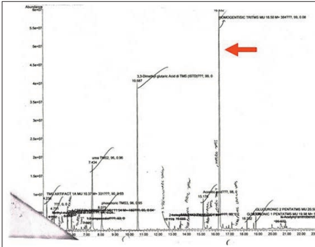
Figure 1: Chromatogram showing Homogentisic Acid Peak (marked with red arrow).
