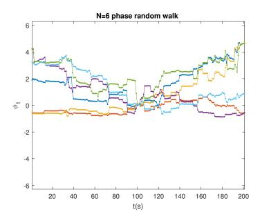
Figure 2.9: Evolution of phase angles of 6 elementary nonlinear coherent components used in the reconstruction. The synchronization of phases occurs at t = 100 seconds, when the extreme wave height is realized.
