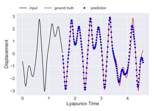
Figure 5.10: Softening forced Duffing oscillator with  $\gamma = 0.5$  prediction (No.3).
