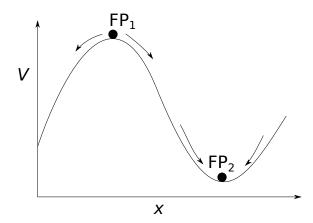
Figure 1.2: Diagram of potential valley of V associated with (1.1) where  $\frac{dV}{dx} = -f(x)$ .  $FP_1$  can roll down from the top of the hill and any perturbation will destabilize the equilibrium;  $FP_2$  lies on the valley and the state x will come back to  $FP_2$  regardless of any local perturbation.
