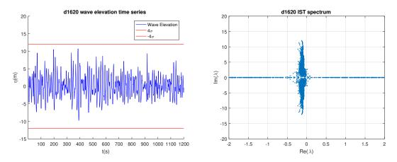
Figure 2.3: Wave elevation time series recording from UTC 16:00 and corresponding inverse scattering spectrum.
