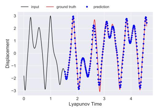
Figure 5.9: Softening forced Duffing oscillator with  $\gamma = 0.5$  prediction (No.2).
