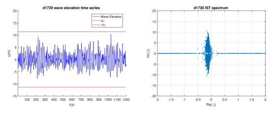
Figure 2.4: Wave elevation time series recording from UTC 17:00 and corresponding inverse scattering spectrum.
