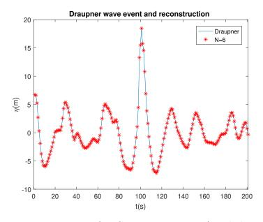
Figure 2.7: Draupner wave event (UTC 15:00, 1 Jan 1995) and the time series reconstruction through the stochastic model of the current work with 6 elementary nonlinear coherent components.
