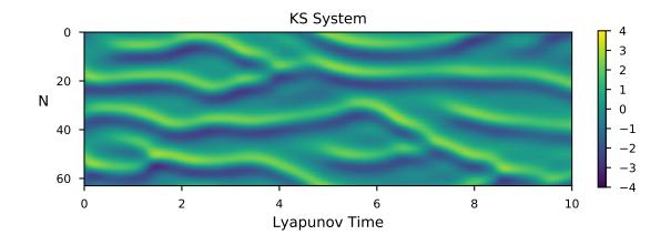
Figure 4.3: Scalar field of the Kuramoto-Sivashinsky equation. Vertical axis is the spatial domain, discretized with the grid size of 64. Horizontal axis shows the non-dimensional Lyapunov time which is the product of the maximal Lyapunov exponent and time. Colorbar denotes the magnitude of the scalar value u(x,t), ranging from -4 to 4.
