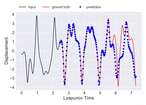
Figure 5.11: Softening forced Duffing oscillator with  $\gamma = 1.7$  prediction (No.1).
