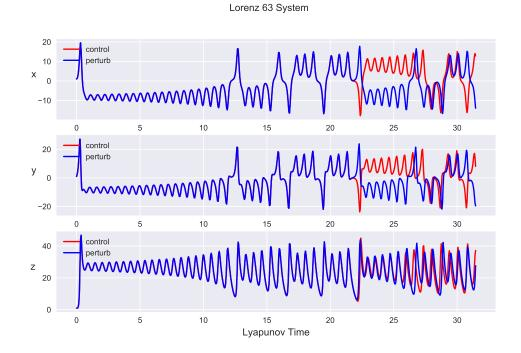
Figure 4.1: x, y, and z component time series of Lorenz'63 system. The two trajectories are initially separated by  $10^{-15}$  units. The divergence is visible after 23 Lyapunov times.
