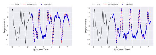
Figure B.20: *left*: Softening Duffing with  $\gamma = 1.7$  prediction (No.6); *right*: Softening Duffing with  $\gamma = 1.7$  prediction (No.7).
