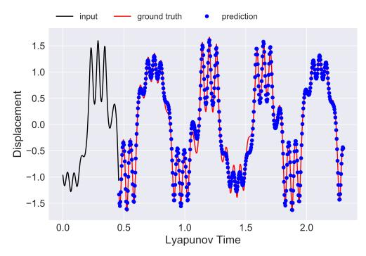
Figure 5.15: Hardening forced Duffing oscillator prediction (No.2).
