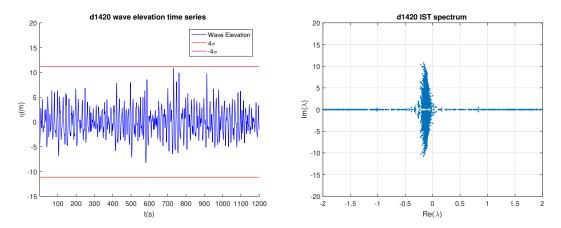
Figure 2.1: *left*: Wave elevation time series during Draupner event recording from UTC 14:00.  $\pm 4\sigma$  (4 times standard deviation)values are shown as red lines to help visualize extreme wave height; *right*: corresponding inverse scattering spectrum calculated from the time series in left panel.
