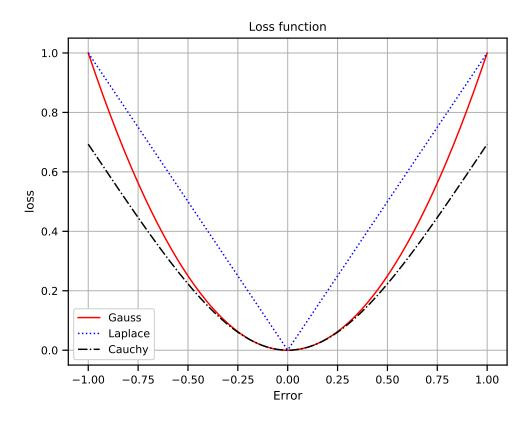
Figure 4.4: Illustration of the variations of three loss functions with respect to the error  $e = \hat{y} - y$ . i) Gauss loss function (red solid line):  $l = e^2$ ; ii) Laplace loss function (blue dot line): l = |e|; and iii) Cauchy loss function (black dot-dash line):  $l = \log (1 + e^2)$ .
