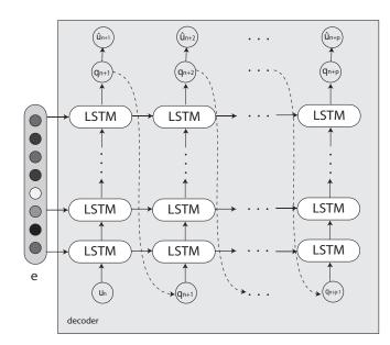
Figure 4.7: Unrolled decoder consists of multiple LSTM layers. The preceding time step output  $u_t$  is used as the input at the next time step. Again, highway connections have been added to help train the deep networks (which are not shown here). The output prediction  $\{\hat{u}_t, n+1 \leq t \leq n+p\}$  is expected to be close to  $\{u_t, n+1 \leq t \leq n+p\}$  after the training.
