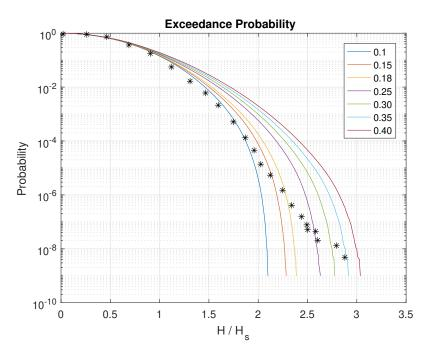
Figure 2.10: Probability of exceeding wave height from simulation of stochastic interference of six waves. Different lines corresponds to different wave steepness  $\epsilon$ , ranging from 0.10 to 0.40. Black stars are used to represent field measurements of freak waves from reference [1].
