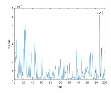
Figure 2.8: Reconstruction residual of the Draupner wave event with 6 elementary nonlinear coherent components.
