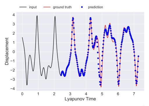
Figure 5.13: Softening forced Duffing oscillator with  $\gamma = 1.7$  prediction (No.3).
