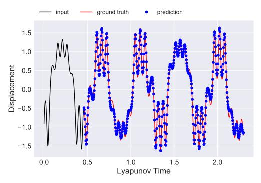
Figure 5.16: Hardening forced Duffing oscillator prediction (No.3).
