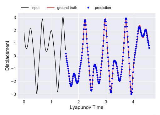
Figure 5.8: Softening forced Duffing oscillator with  $\gamma = 0.5$  prediction (No.1).
