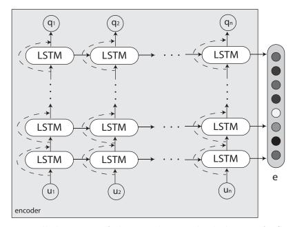
Figure 4.6: Unrolled version of the encoder. Multiple layers of LSTM cells are stacked in order to extract higher abstractions of the input  $u_i$ . The hidden state  $h_t$  is the concatenation of all hidden states of all LSTM cells. The record vector  $\mathbf{q}_t$  is the output of the top-layer LSTM cell. The thought vector  $\mathbf{e}$  is the final state of stacked LSTM cells. The dashed lines are the highway connections that allow the residual to be passed via a gating mechanism.
