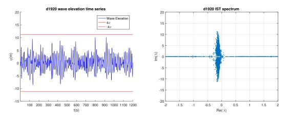
Figure 2.6: Wave elevation time series recording from UTC 19:00 and corresponding inverse scattering spectrum.
