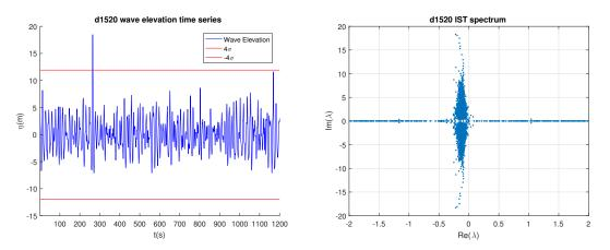
Figure 2.2: Wave elevation time series recording from UTC 15:00 and corresponding inverse scattering spectrum.
