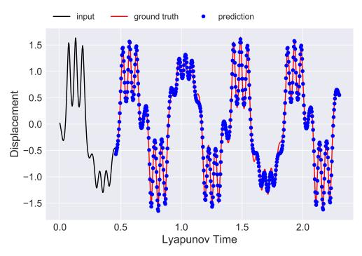
Figure 5.14: Hardening forced Duffing oscillator prediction (No.1).
