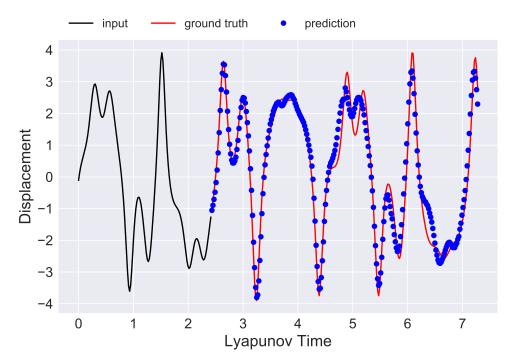
Figure 5.12: Softening forced Duffing oscillator with  $\gamma = 1.7$  prediction (No.2).
