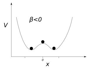
Figure 5.2:  $\beta < 0$  with double potential valleys for unforced Duffing oscillator. Fixed point are located at  $x = 0, \pm \sqrt{-\beta/\alpha}$ . As explained before, the center fixed point is unstable and the other two are stable.
