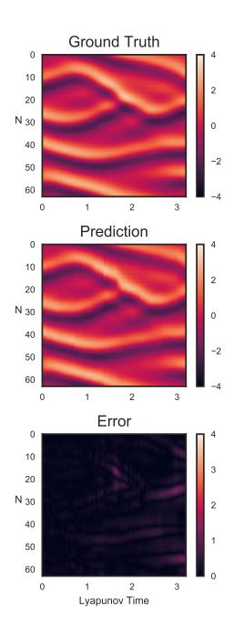
Figure 4.15: KS prediction (No.1). *upper*: true scalar field up to 3.2 Lyapunov times; *middle*: predicted scalar field; *lower*: absolute error as the difference between the true field and the predicted field.
