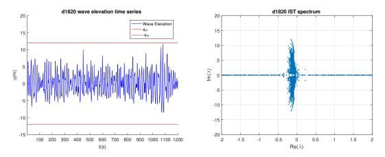
Figure 2.5: Wave elevation time series recording from UTC 18:00 and corresponding inverse scattering spectrum.
