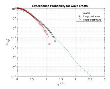
Figure 2.11: Exceedance probability for wave crests from simulation of stochastic interference of six waves. Black stars and red circles represent experimental data from reference [2].
