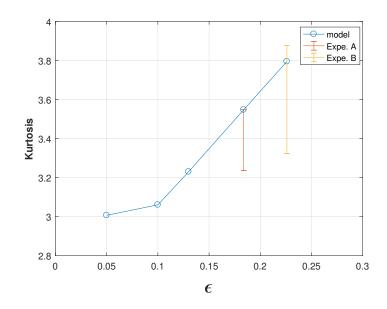
Figure 2.12: Kurtosis of probability density function from the simulation of stochastic interference of six waves with different initial wave steepness. Error bar data are from experiments [3].
