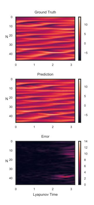
Figure 4.12: Lorenz'96 prediction (No.1). *upper*: ground truth simulation results obtained by solving (4.12) for 3.2 Lyapunov times with N = 48 and F = 8; *middle*: prediction results from the neural machine for the same initial condition; *lower*: absolute error between the ground truth and the prediction.
