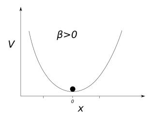
Figure 5.1:  $\beta > 0$  with single potential valley for unforced Duffing oscillator. Fixed point is located at x = 0.
