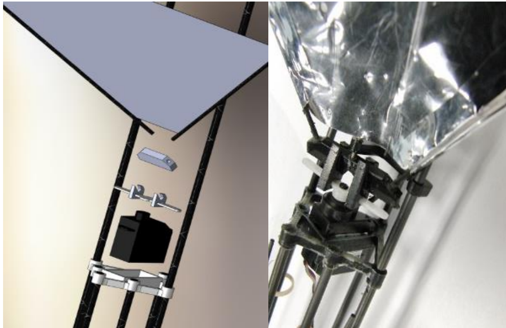
Figure 3.3: Exploded view of tail subassembly (left) and as-built tail (right)
