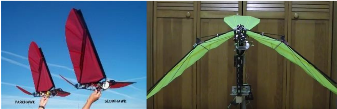
Figure 2.4: Sean Kinkade’s Park Hawk and Slow Hawk ornithopters (left) and a Slow Hawk 2 modified with articulated wing turning (right) [36, 37]
