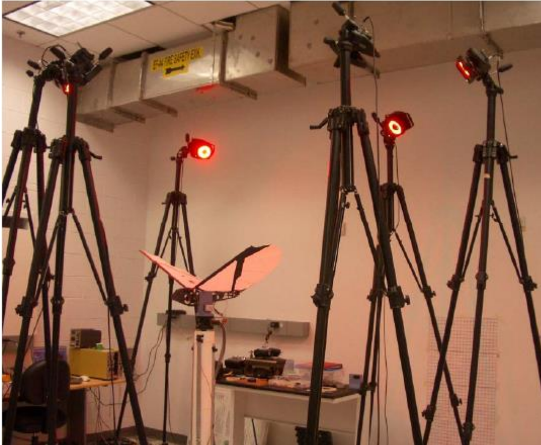
Figure 2.11: Combined VICON and load cell testing conducted at University of Maryland Morpheus Laboratory [25]
