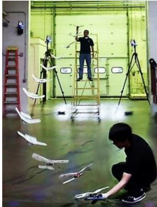
Figure 2.6: Wing-based steering used to perch from the University of Illinois' Aerospace Robotics and Control Group [20]
