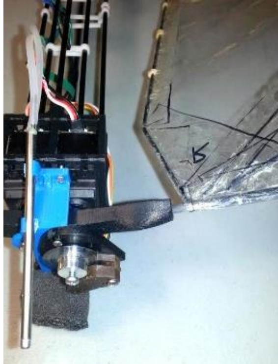
Figure 4.22: Front view of instrumented Robo Raven FWAV showing optical encoder and Pitot tube
