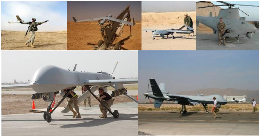
Figure 1.1: Current DoD UAS. Top row, left to right, Raven, ScanEagle, Shadow, Fire Scout. Bottom row, left to right, Predator, Reaper [4-9].
