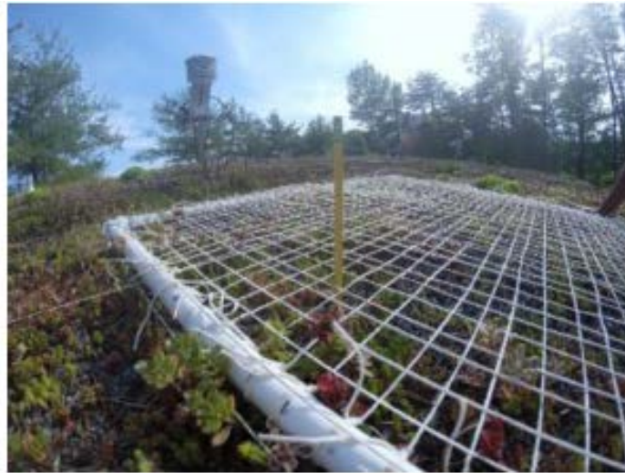
Figure C-2 Grid pattern used for measuring LAI, 1m x 1m in size.
