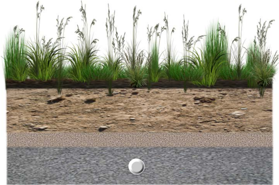
Figure 2-4 Surface runoff and stormwater runoff flowing from the constructed wetland flows into a 32.6 m 2 bioretention (7.62 cm mulch layer, 70.0 cm planting media, 15.2 cm sand layer, 15.2 cm stone layer above the underdrain, and 7.62 cm stone layer below the underdrain) with groundwater outlet. Plant list and media specifications were not accessible.
