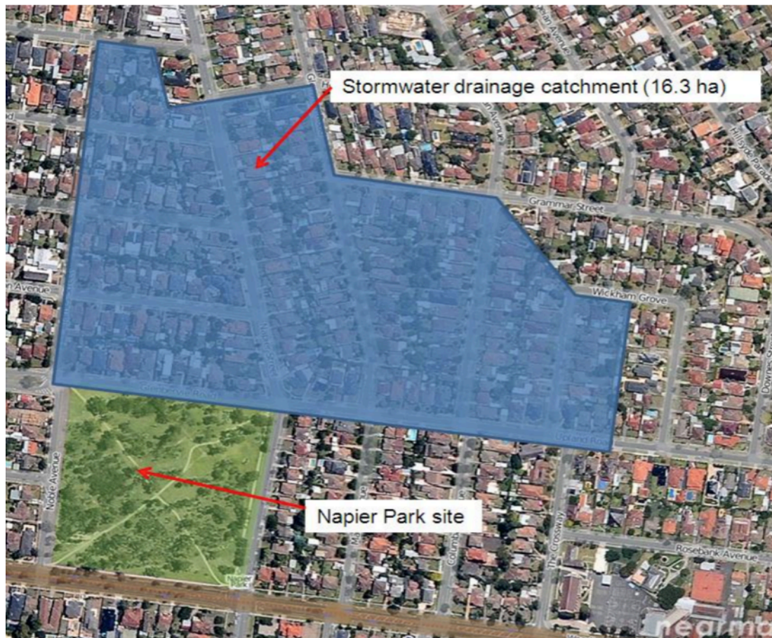
Figure 15: The layout of a storm drain harvest and cistern storage system shows the stormwater collection area and area to be irrigated using the harvested stormwater (AECOM Australia Pty Ltd., 2010).
